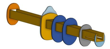
First, Using the A-Fold technique first used by Flite Test, assemble the Center Pod, then glue on all of the formers using the corresponding marks on the Center Pod.
