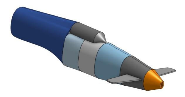
Pass the Canard through the opening in the skin and center pod, trim with a knife if needed. Glue it on the edges.
