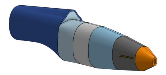
The Nose Skin is a bit different because it will be open at the end with no former or skin to fill the hole, a 3d printed nose will be added later on. If you don't have a 3d printer or have no access to one, you can simply sand a piece of pink insulation foam to shape.
