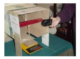
The fan used in this experiment was a three speed version. Nine readings were taken with a wind speed indicator, at each of the fan speeds. The following table summarises the results.
