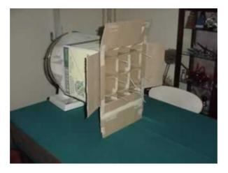
A test of the airflow at this stage showed some dead air spots on the sides and bottom of the airstream, and so these passages were blocked off at the end away from the fan itself.
