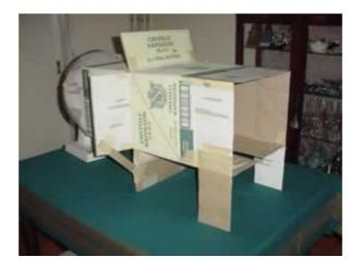
Before testing any wing sections, check that the airflow at the shroud exit is reasonably straight and even. To do this use a tissue streamer taped to a skewer, and move it around in the airstream. Dead areas within the airstream will show up with the streamer hanging down limply.
