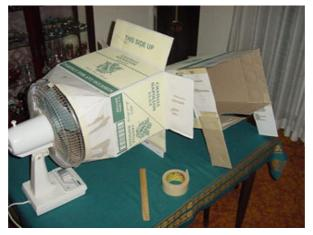
The bottom flaps of the second box were lined up with the sides of the box to extend the tunnel shape to 700 mm. A slot was cut in the bottom flap  $(30 \times 150 \text{ mm})$  to allow the test mounting stand to sit in the airstream about 100 mm from the end of the tunnel shroud.
