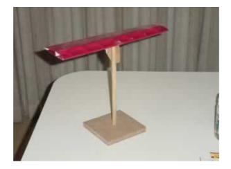
A piece of balsa sheet was cut to a semicircular (protractor) shape and glued to the underside centre of the wing section to mount the wing to the test stand. A pivot hole was drilled and a scale in 5 degree increments was added from -10 to +30 degrees of angle. Zero degrees was equal to the bottom of the wing section being horizontal.
