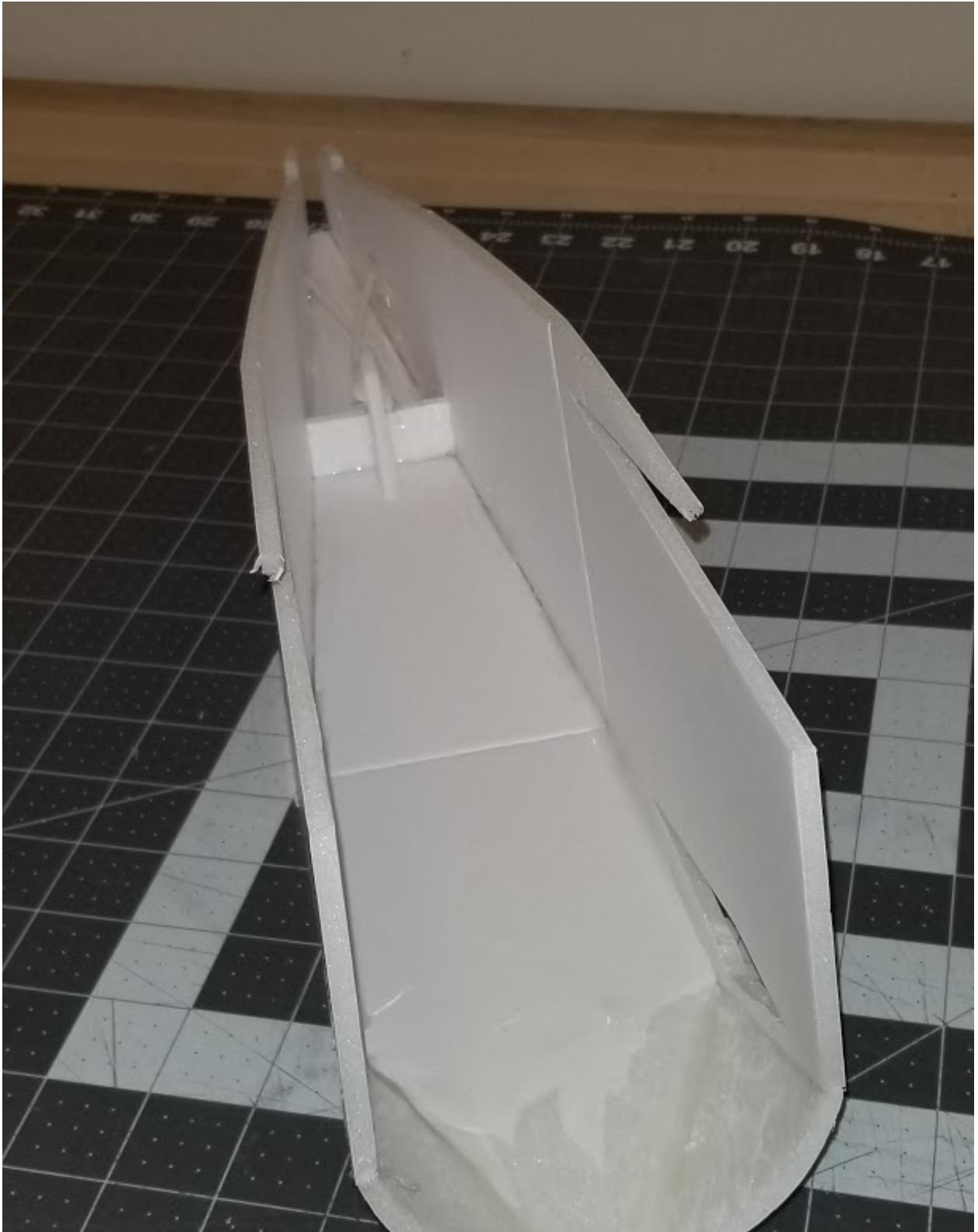
Tail linkage Guides Installed
