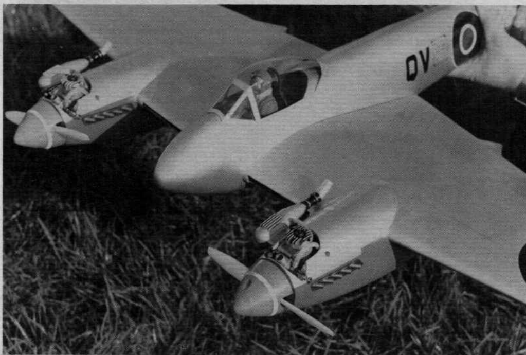
ABOVE: Prototype with O.S. .10s installed. Note muffler extensions to blow exhaust away from wing. LEFT: Hornet rests on its dolly. This is used when a smooth runway is available.
