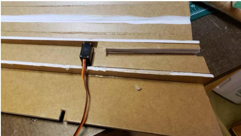
Cut a notch in the spar so that the servo leads can pass into the space behind the spar. Then pass the servo leads through the servo hole in the wing and into that slot.
