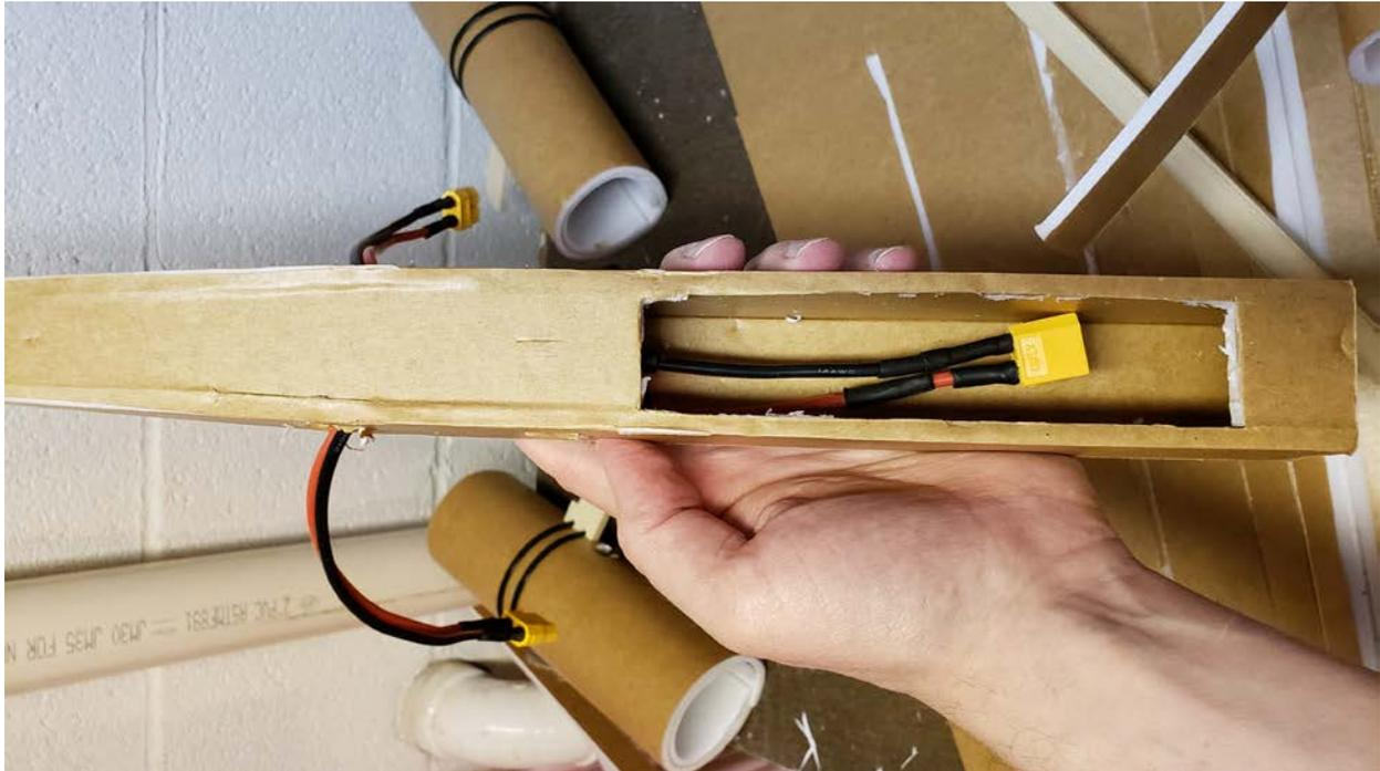
To get the battery extension from the hatch out into each wing, I ended up pulling the “square” portion of the fuselage out of the cylindrical portion and passing them through, the passing them through the cylinder as I slid them back together.
