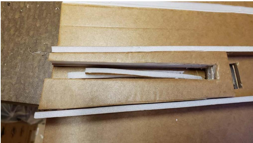
Insert the spacers that hold the wood dowel in the spar. The narrow side goes toward the front of the wing. Trim as needed so that the wood dowel fits snugly into the slot.
