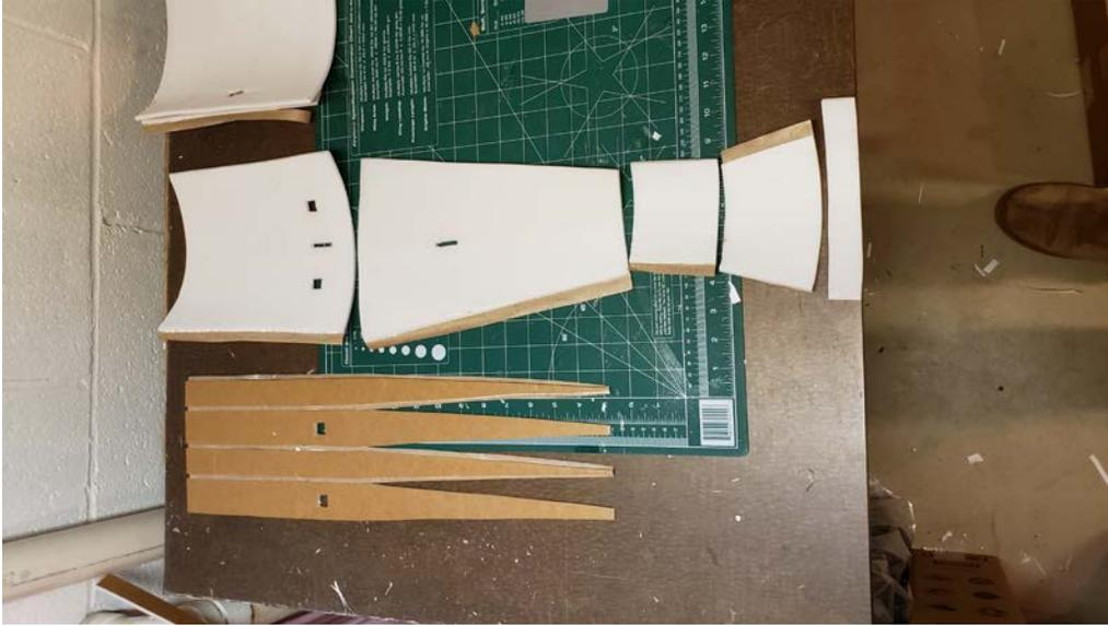
Fold & glue the fuselage center with B folds. Enlarge the rectangular hole in the top of the front enough that your battery will sit in it and rest on the bottom. I enlarged the hole toward the front.
