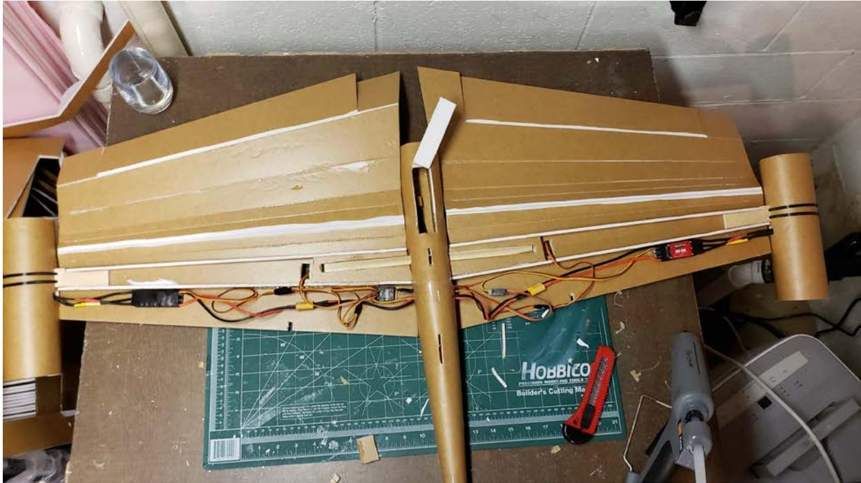
I extended the ESC and servo leads from the right wing through the fuselage to the left. That allowed me to put the receiver in the left wing, behind the spar. I had to cut a hole for it in the lower portion of the wing. That actually let me pull it out and trouble shoot my ESCs after my maiden crash, so I would do it again.
