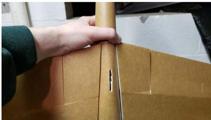
Where the top wing meets the “bat” will require some trimming. I then glued that piece and the fixed portion of the wing near the EDF pod level with the midline of the fuselage.
