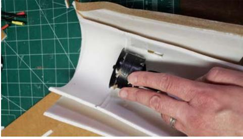
Place the EDF into the inner EDF tube. You want the EDF “body” to sit where the rectangular hole is for the plywood spar extension to rest on it. The square hole goes toward the rear for the leads to pass through. Wrap the inner and outer EDF tubes together around the EDF, and use packing tape to hold them.
