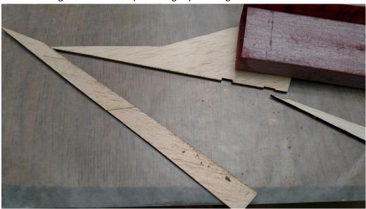
There is a slight angle on the dihedral gage at the pointed end. Use this to set the gull dihedral of the inner panels as you join them to the outer panels. Make sure that you mirror the wings so that you do not end up with two left or two right wings!
