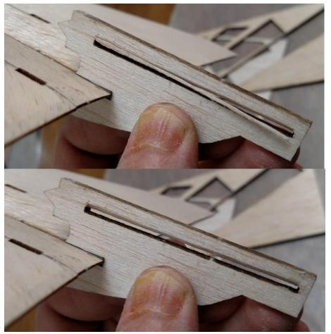
Insert the tail assembly and glue it in place.
