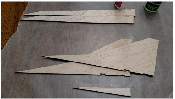
Bevel the wing inner and outer panels slightly for the gull dihedral.
