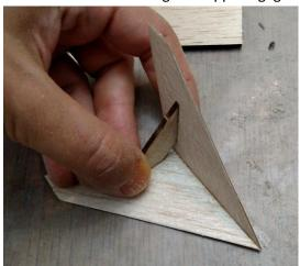
Use a razor blade to bevel out the slot for the tail fins.
