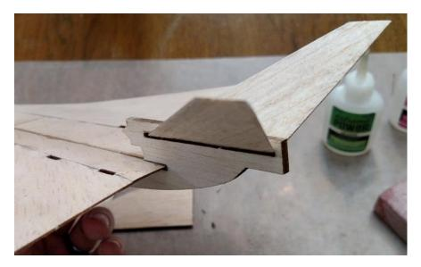
Separate the 1/8" balsa engine nacelles and bevel the top keys so that they will fit into the slots in the wings.
