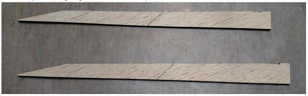
Separate the 3/32" balsa wing outer panels and the dihedral gage.
