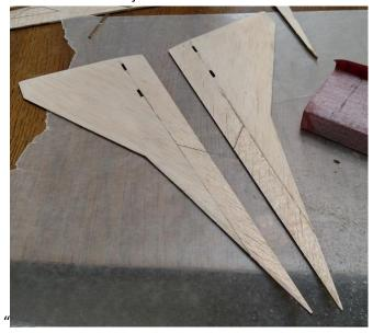
Use the dihedral gage to set the slight dihedral between the two panels as you cement them together with CA glue. The slight bend that is included for the gull dihedral should nest against the outer dihedral
