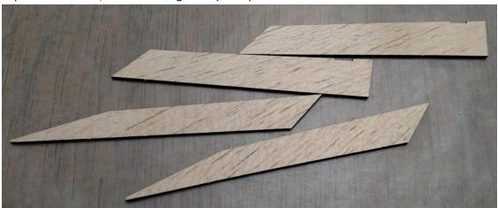
Join these pieces using CA glue to form the inner panels.
