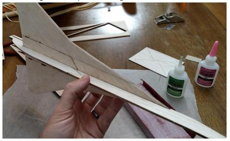
Remove the 1/32" balsa tail fins from their carrier sheet.
