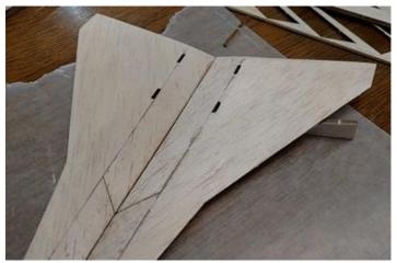
Glue the wing onto the top of the fuselage as shown below.
