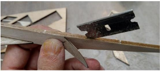
Press the catapult hook at least 1/8" into the slot and glue it firmly in place with thin CA.
