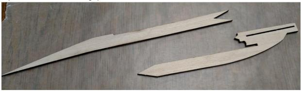
Use CA glue to join the fuselage halves together over wax paper. Do this on a flat surface to ensure the fuselage is straight.
