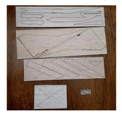
Separate the 1/8" balsa fuselage parts from their carrier sheet as shown below.
