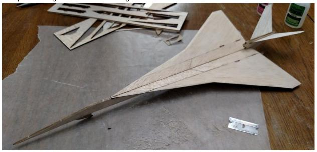
I found that the model needed a the wingtip trailing edges bent up about 1/32" to achieve a stable glide combined with bending the tail fins up about 1/16". This is only an estimate; you will have to tweak the model's incidence and CG settings some to get a glide that meets our flying style.
