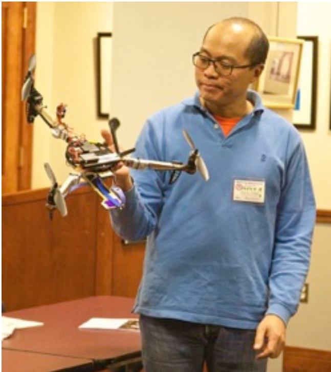
Dave Mak showed a tricopter made primarily with Flite Test structural components. The craft uses a FR Sky receiver and an 8-bit Flip flight controller. This model is for line of sight operation at the moment and has no FPV or navigation systems.
